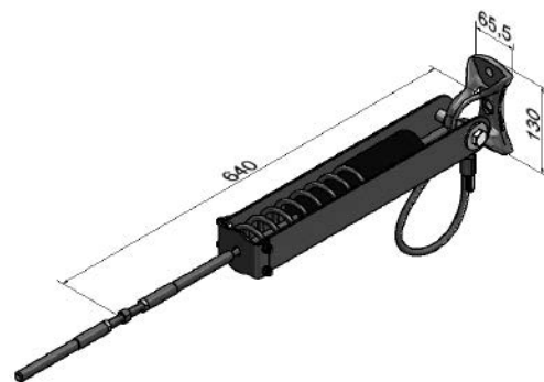
Fig. 18. LDV053 Anchor with absorber and turnbuckle.
