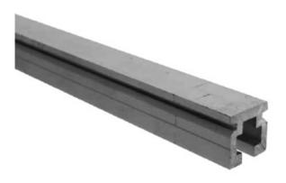
aluminium Al Mg Si 0.5 with anodization treatment to prevent electrolytic corrosion between the steel structure and the rail Can be painted any desired RAL colour.
